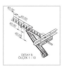
Note: The chassis can be extended by 240 mm at the front and 240 mm at the rear, with 60 mm increments, allowing a total extension of 480 mm.
